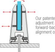
Our patented 3-point panel adjustment system allows for forward-back and angular alignment of the glass panel.
