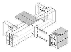
**JH Clamp** can be used to create hidden fixing decks for the ultimate seamless design.
