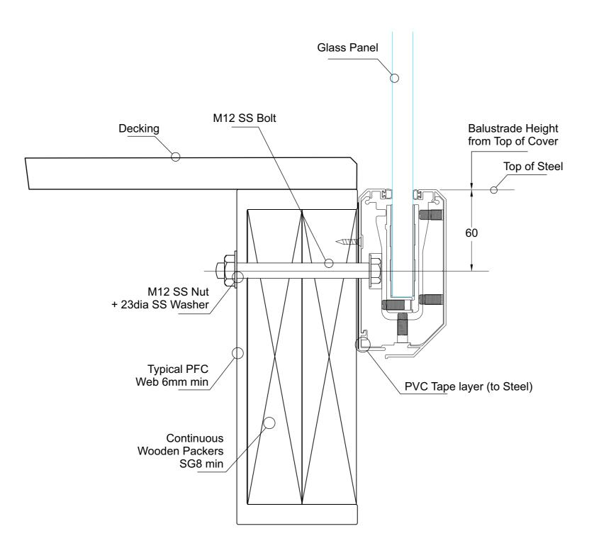
Typical Face Fix to Steel + Wooden Packers - M12 SS Bolt
