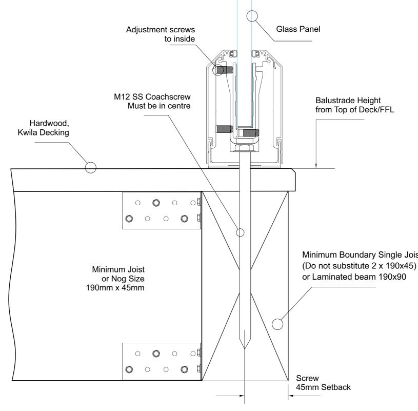
Minimum Boundary Single Joist size 190mm x 90m
