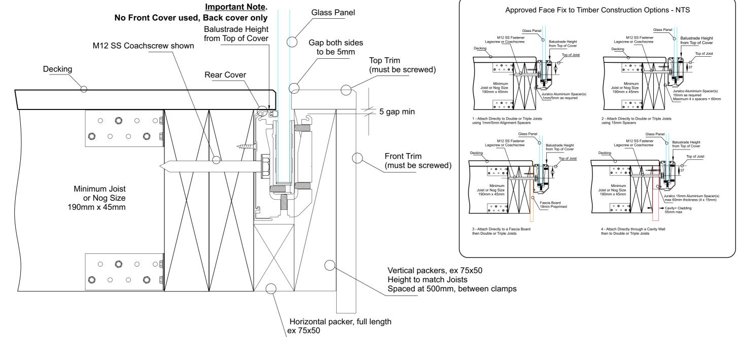
Typical Face Fix to Triple Joist Timber - M12 SS Coachscrews
