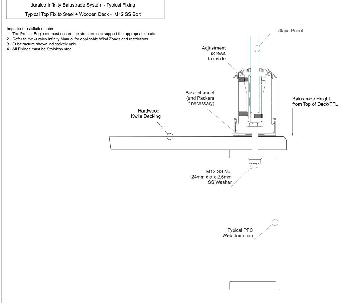
Typical Top Fix to Steel - M12 SS Bolt
