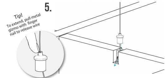
Thread wire a few inches through Adjustment 3. Insert wire through adjustment 4. Screw both adjustments till tight.
