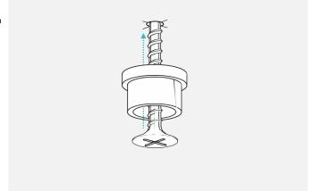
Insert supplied screws\* into adjustment 1 and screw into ceiling at marked spots.
