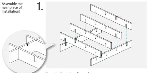
Place 2 x (Part 1) on flat surface. Align 4 x (Part 2) perpendicular to part 1. Slide into all slots until flush.
