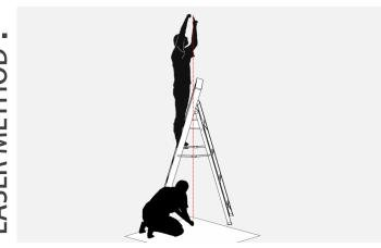
Lay supplied stencil on ground directly below ceiling surface you would like to install your Vista panel.
