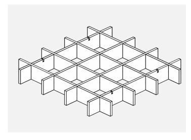
Finished baffle without wire attachment.
