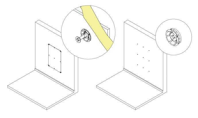
2 With stencil taped to the wall, screw a male Ready clip into each hole.
