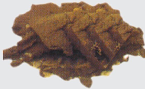
Polyester foam breaks down from hydrolysis, polyether foam should always be used in areas subject to heat and humidity
