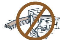
DO NOT lift I-Joists whilst they are lying flat. Excessive flapping may cause damage.
