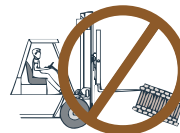
DO NOT lift or roll I-Joists by the top flange.
