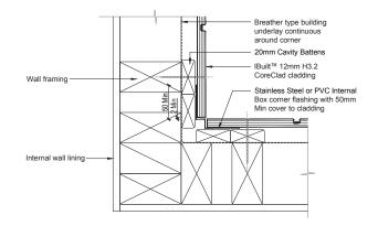
2.3 CoreClad™ Window Jamb Detail Line of head flashing over Joinery as per Arch spec Flexible flashing tape to sill and extended 100mm min up M ajął jambs and 50mm min onto wall as per Fig 72A E2/AS1 80 Y a Continuous protective selant 5 Min Wall framing at over foam bond breaker iamb 20mm Cavity Battens Breather type building underlay to E2/AS1 Internal wall lining IBuilt™ 12mm H3.2 CoreClad cladding
