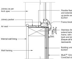
Flexible flashing tape to sill and extended 100mm min up jambs as per Fig 72A E2/AS1
