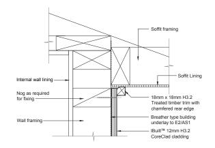
CoreClad™ Soffit Junction
