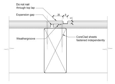
Do not fix through the top lap or weather groove of the shiplap.
