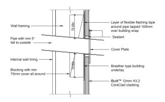
IBuilt™ CoreClad Ply Cladding is to be installed as per the requirements of Clause E2/AS1 Section 9.8 13
