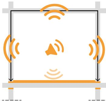
The floor assembly reduces noise propagation through the ceiling. The use of resilient decoupling profiles reduces the propagation of airborne and structural noise.
