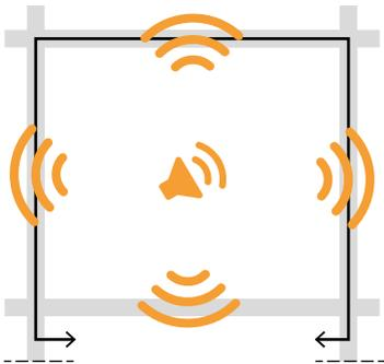
Airborne noise is transmitted to adjacent rooms either by air or by structure, following the paths represented by the arrows (lateral transmission).
