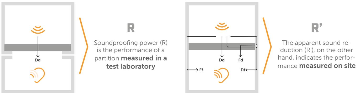
The acoustic laboratories are constructed in such a way that the chambers are completely decoupled from each other, so that lateral transmissions are completely eliminated. **For the same construction assembly and installation, the performance measured in the laboratory will therefore be better than the performance measured on site.**
