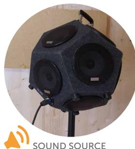
The measurement is performed by activating a specific noise source in the emitting environment and measuring the sound pressure levels in both environments (emitter and receiver). The sound reduction is given by the difference of the two measured levels. Therefore, the higher the  $R_w$  value, the better the acoustic performance of the construction assembly.
