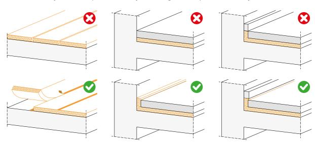
The resilient layer must be continuous because any gap would represent an acoustic bridge. When installing underscreed mats, care must be taken not to create discontinuities
