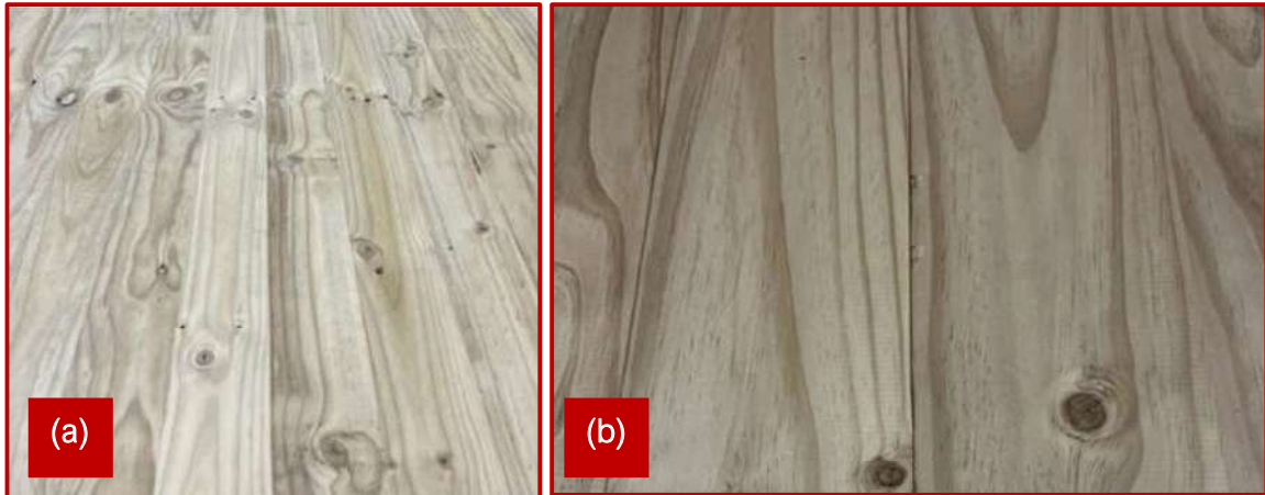
Figure 146: Red Stag H3.2 treated EWP panels generating a slight green tinge; a) Open View; b) Close View.
