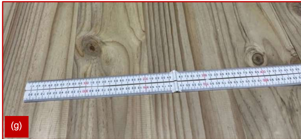
Figure 142: Example of knots, wane and knot voids in Standard (Non-Visual) Grade of CLT panels.
