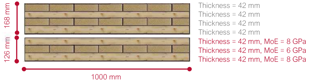
Figure 115: Red Stag CLT Panel Cross-Section
