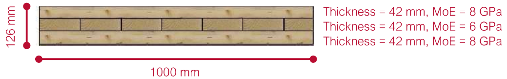
Figure 109: Red Stag CLT Panel Cross-Section
