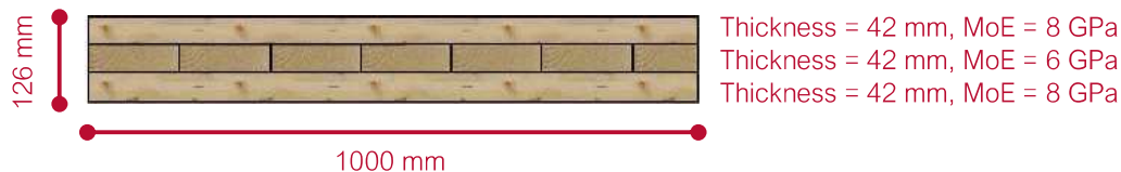
Figure 117: Red Stag CLT Panel Cross-Section
