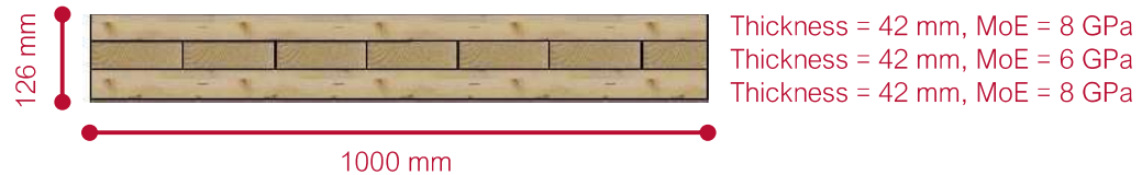
Figure 107: Red Stag CLT Panel Cross-Section
