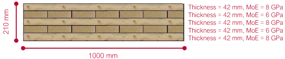
Figure 111: Red Stag CLT Panel Cross-Section
