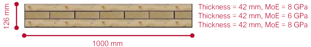
Figure 119: Red Stag CLT Panel Cross-Section
