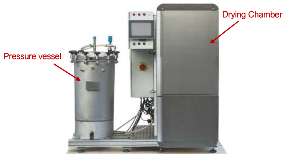
Figure 86: Delamination testing equipment.
