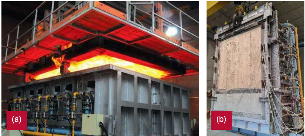
Figure 91: Large-scale fire testing on Red Stag EWP conducted by BRANZ; (a) Red Stag CLT floor test specimen after fire testing; (b) Red Stag CLT wall test specimen before fire testing.
