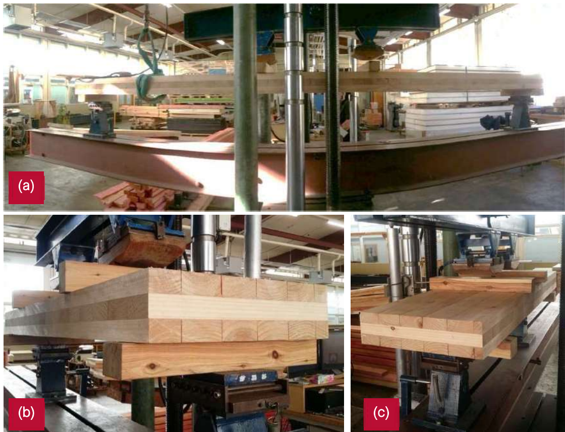
Figure 89: Large scale mechanical testing conducted by SCION; (a) Long span testing; (b) Medium span testing; (c) Short span testing.
