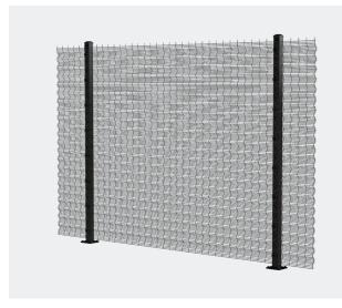
**Ngarumesh 358 is the same cost as tubular steel or aluminium fencing** but offers much higher security. Absence of horizontal rails reduces the climbing risk and increases visual penetration for security cameras.
