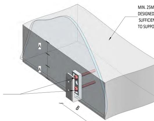
MIN. 25MPA CONCRETE MIN. 190mm THICK
