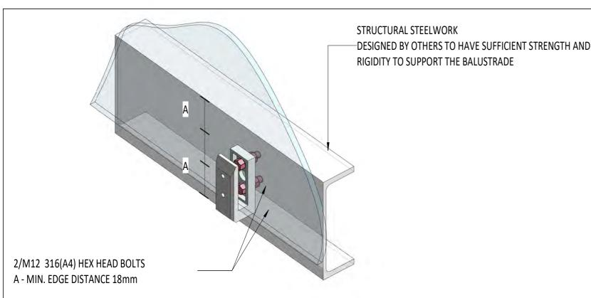
SEPARATION BETWEEN BOLT HEAD AND GLASS TO BE MAINTAINED.
