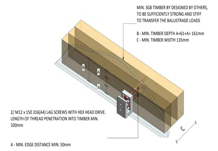
SEPARATION BETWEEN BOLT HEAD AND GLASS TO BE MAINTAINED.
