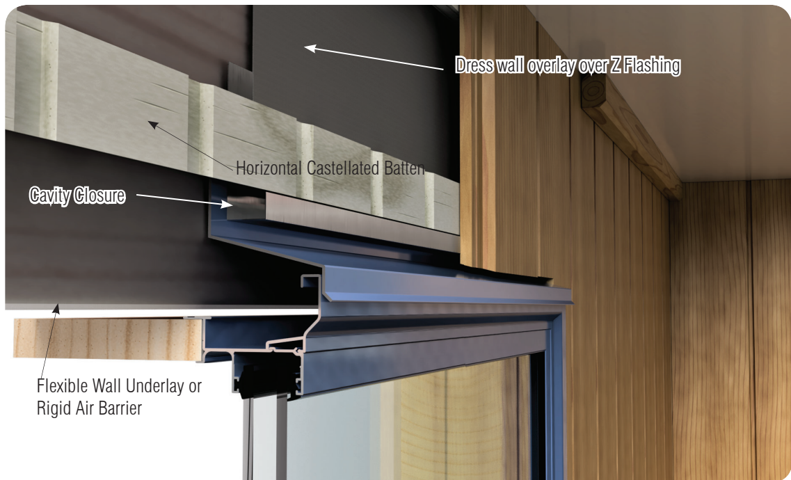
Typical Window and door Detail
