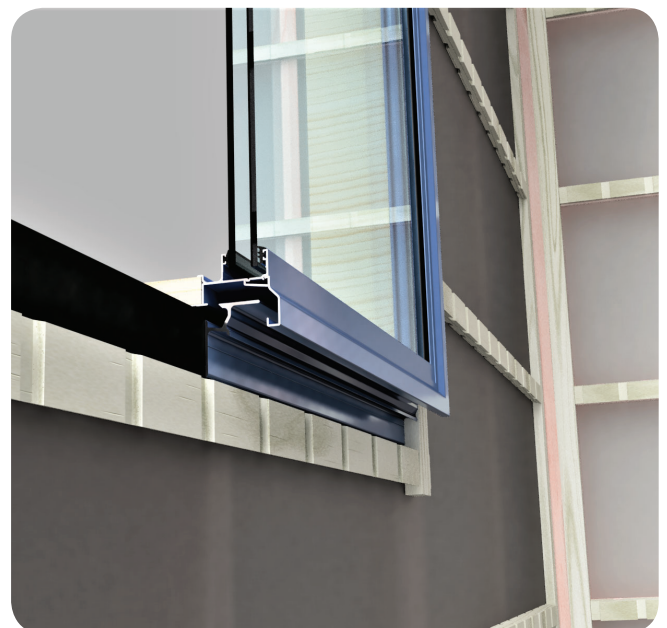
Typical Window Head and Sill Batten layout
