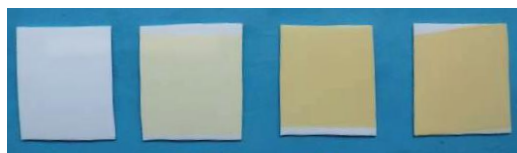
The colour difference of Competitor 1 Cowl over a period of 0 to 5 years.
