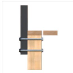
Side fixed to timber deck
