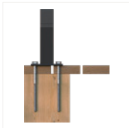
Top fixed to timber deck
