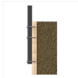
Side fixed to single board retaining wall
