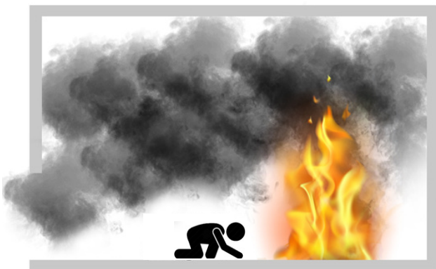
Fig. 1 - fire breaking out in an unprotected room (i.e. without smoke ventilation) will rapidly fill the room with smoke. Occupants can be disorientated and overcome by the heat and toxic gases, and firefighters are forced to work under reduced visibility.
