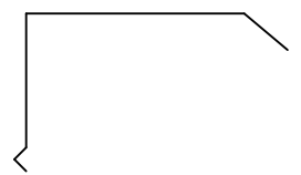
ROOFING INDUSTRIES BARGE FLASHING
