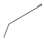
ROOFING INDUSTRIES GUTTER APRON FLASHING
