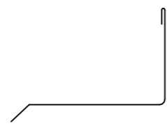
ROOFING INDUSTRIES APRON FLASHING
