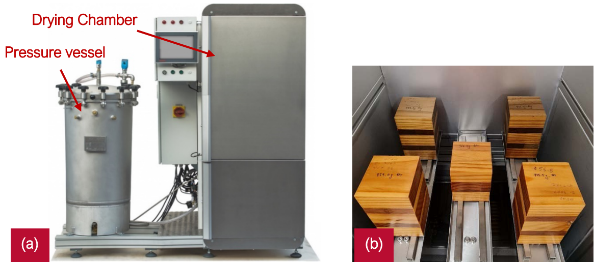
Figure 15: Red Stag CLT quality assurance; a) EWP delamination testing equipment; b) CLT specimens for delamination testing.
