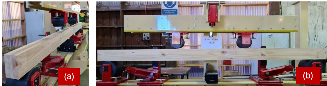
Figure 3. Large-scale mechanical testing of Red Stag CLT beam conducted by Red Stag; a) End Elevation; b) Elevation.
