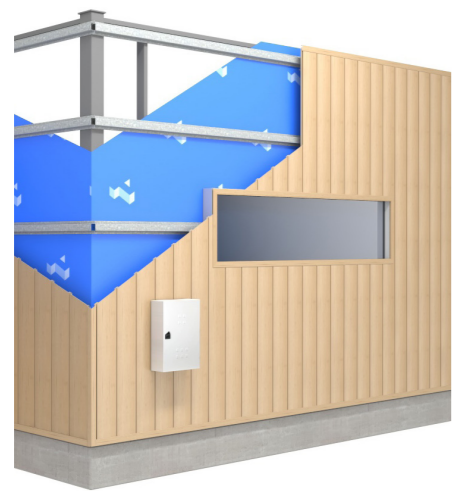
Cladding - Vertical Over Top Hats
