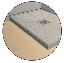
Fix a 10x50mm Expansion Joint Foam Tape to the Shower Tray Module, ensure there is a 20mm distance from top of the foam to the top of the shower tray.
