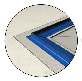
Apply Waterproof Sealant generously to create a bond breaker on both sides of the aluminium angle, tool the sealant to create a min. 3-5mm radius.
