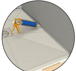
• Apply a continuous 6-8mm bead of the waterproof sealant at the joint between Shower Tray Module and Wet Area Lining.
