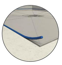
Seal the gap between the Shower Tray Module and Maglok Dragonboard entirely with Flexible Joint Sealant until it reaches the Expansion Joint Foam Tape.
