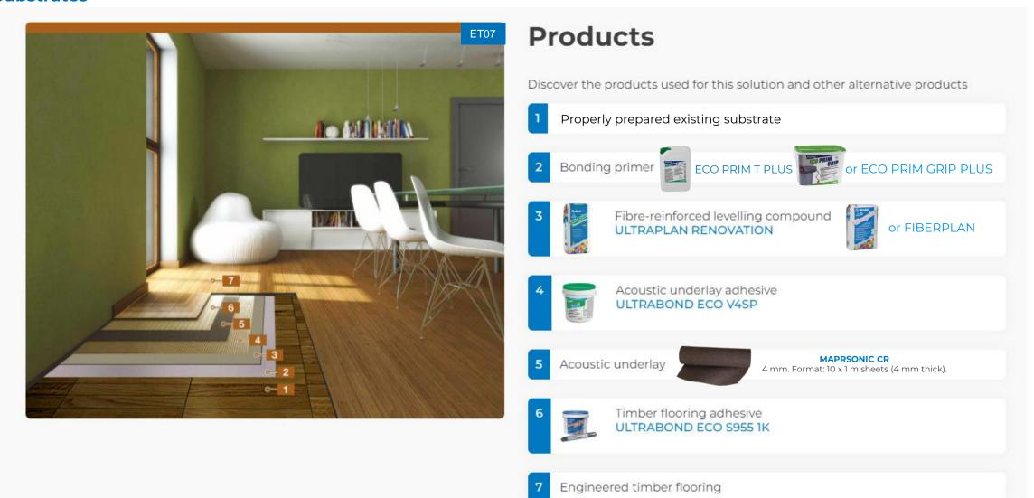
For composite timber; fiber cement; other/difficult ie. Magnesium oxide, ridged extruded polystyrene foam, texisting ceramic, stone and terrazzo substrates.
