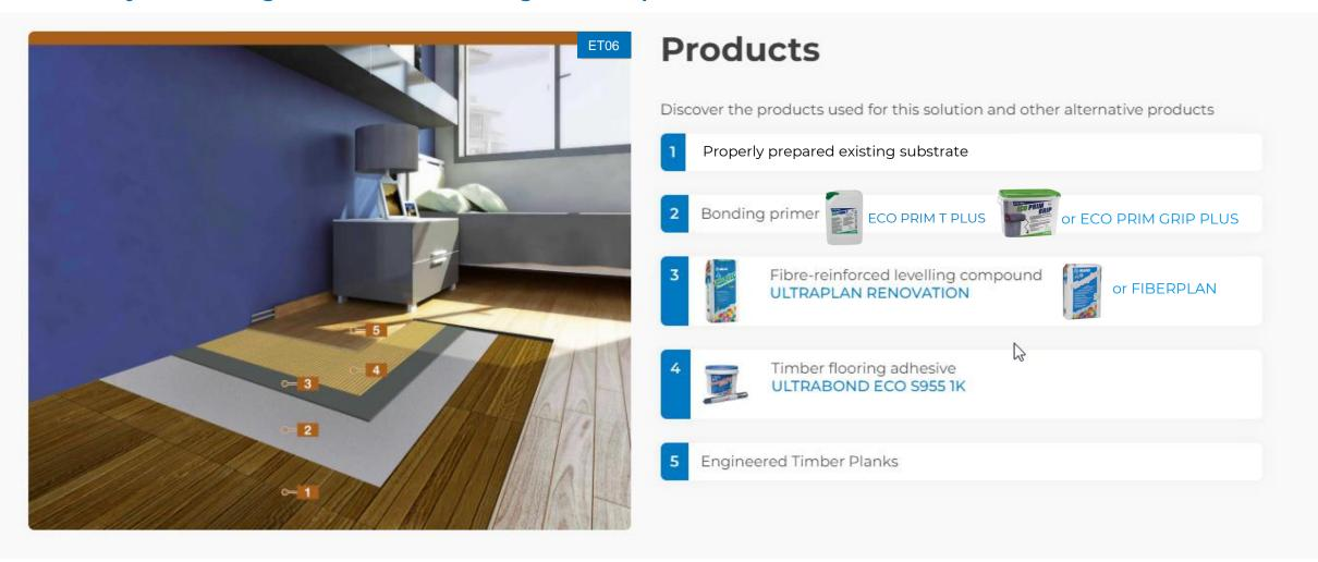
For composite timber; fiber cement; other/difficult ie. Magnesium oxide, ridged extruded polystyrene foam, existing ceramic, stone and terrazzo substrates.
