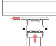
SL-RCA180 slides into profile groove, SL-RCF90 into profile end, fastens with supplied grub screws.
