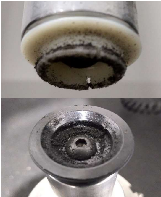
Figure 4 - Pull-out test after 500 cycles
