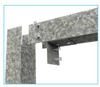
The vertical C-track is cut away at the top. The horizontal C-track is cut so that a flap can be folded down and screwed to the vertical C-track.
