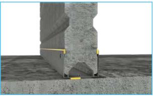
16 Fire rated sealant details for top, bottom and sides
