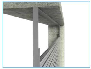
Keep placing the panels and fixing them to the panel below.
