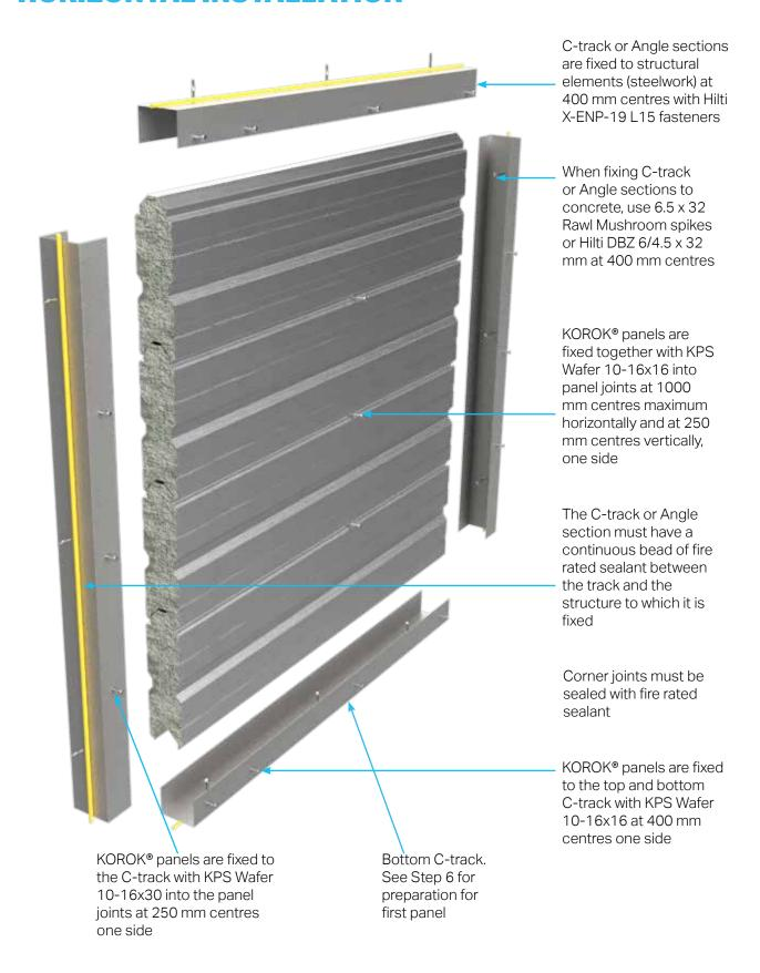
Horizontal Installation of the KOROK® panels requires the C-track to be fixed to the supporting structure, e.g. walls, columns, portals etc.
