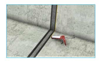
For horizontal installs where the wall width is greater than 5.0m OR where the load is transferred to the ground (e.g. 4-sided plant room), grout or a panel nose must be used in the bottom C-track.
