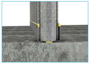
15 Using Angle as an alternative to C-track.
