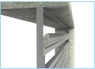
Once the last panel is in position, fix the pieces of C-track that were removed in Step 10, back in place. Fire-rated sealant is then applied.
