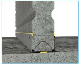
KOROK® panels must be cut 30 mm shorter than the structural opening measurement to allow for fitting.
