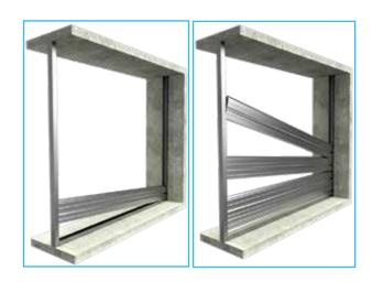
Ensure the panels are clicked together correctly to maintain the fire and acoustic performance. Remove strippable film at the end of each day's work.
