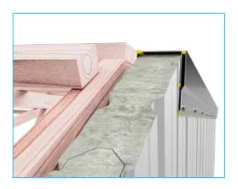
Install a KOROK® KIT flashing over the mid-wall joint fixed at 250mm centres top and bottom using KPS Wafer 10-16x16 screws.
