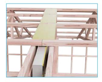
Once the top chord on the second side is completed, fix KOROK® aluminium brackets into the panel joints at 500mm horizontal centres and a maximum of 3.0 metre centres vertically.
