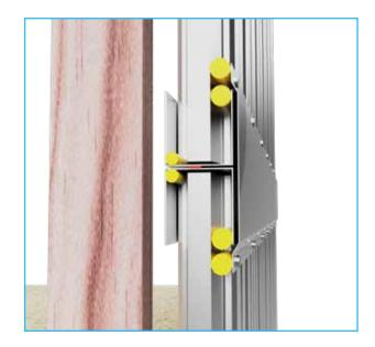
Ensure the wall is screwed off at each panel joint on one side at 1000mm centres vertically with KPS Wafer 10-16x16 screws. The horizontal bottom and mid-wall C-track is screwed off to the KOROK® panel with KPS Wafer 10-16x16 screws at 250mm centres one side.
