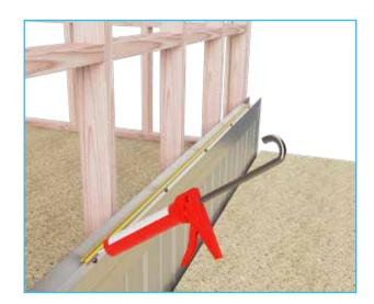
Fix the vertical C-track to the first panel using KPS Wafer 10-16x16 screws at 400mm centres one side, prior to installing. Place fire rated sealant in the internal corner of the vertical C-track.
