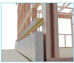
Place a bead of fire rated sealant on top of the C-track.
