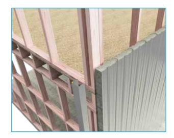
Ensure the wall is screwed off at each panel joint on one side at 1000mm centres vertically with KPS Wafer 10-16x16 screws.
