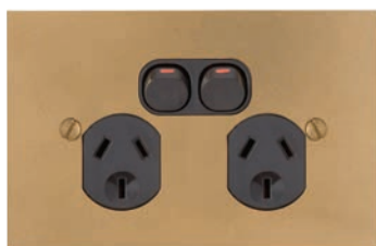
BBSL25A Twin Switched Socket Outlet 250V, 10A Cut out: 77mm L x 57mm W
