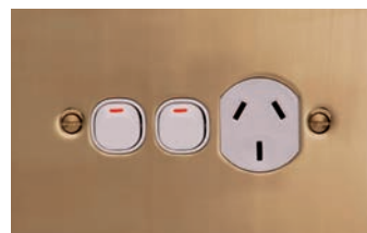
BBSL15XA Single Switched Socket Outlet, with extra removable switch 250V, 10A Cut out: 76mm L x 53mm W.
