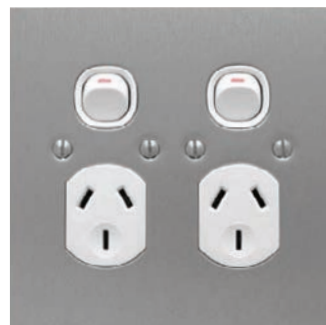
B15V2A Twin Switched Socket Outlet 250V, 10A Flat Plate 115mm L x 115mm W Cut out: 112mm L x 73.5mm W
