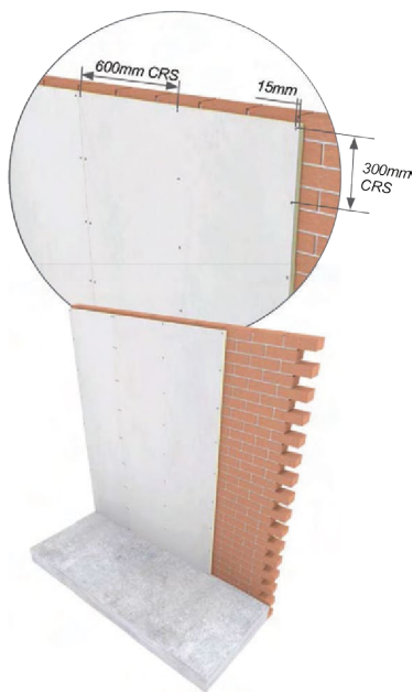
Figure 1.6. Masonry brick or block wall
