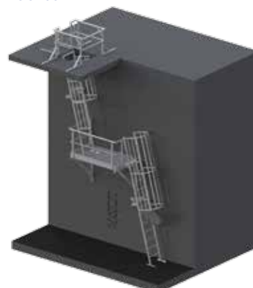
LD35 ANGLED CAGE LADDER WITH MIDWAY LANDING PLATFORM - INTERNAL ACCESS
