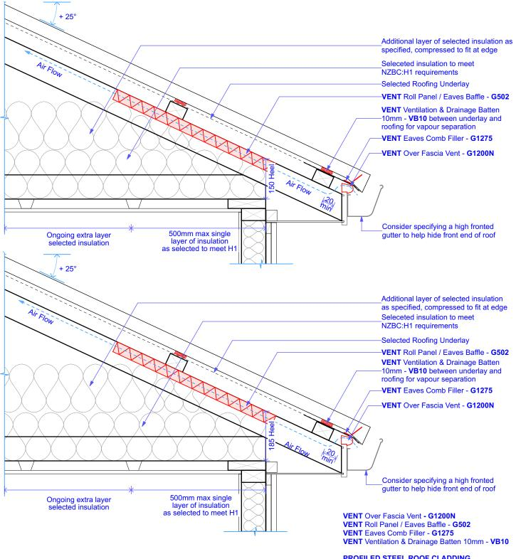
PROFILED STEEL ROOF CLADDING Ventilated Fascia - Roof Eave - 25° (10,000mm<sup>2</sup> lin/m)
