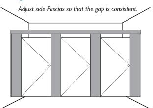
Repeat for the remaining doors. Once gaps are consistent, fix the last Fascia. **Use (B) 8GA x 12 screws.**
