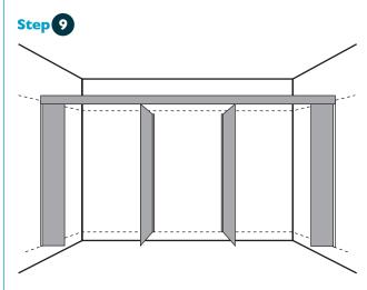
Trim the Headrail to ensure flush with the walls and position on to the top of the Side Fascias.
