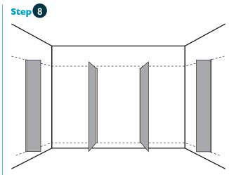
Place hinged Fascia into side U-Channels and align at the bottom. Ensure Plumb, and then fix on the inside of the cubicle with 4 Rivets, 30mm and 600mm down from the top, and the same up from the bottom.
