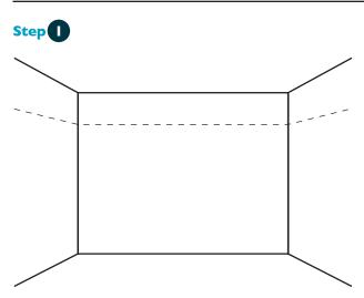
From the plans, mark Datum on relevant walls. Ensure that the lowest point in the floor is used for Datum otherwise the system could be on an angle, or the Headrail height could be too low.
