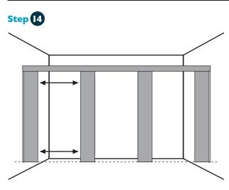
Starting with the Hinged Side Fascia, ensure that the door gap at the bottom is the same as the top gap.
