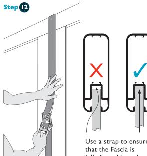
Use a strap to ensure fully forced into the Headrail pocket.
