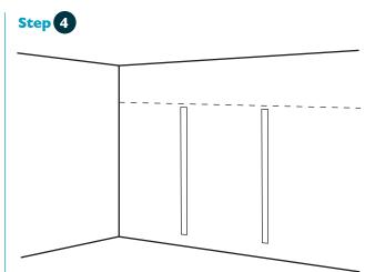
Fix back U-Channels (1748mm) centred on your marks, 47mm below the Datum line. The U-Channels are predrilled. Ensure screws go into wall frame.
