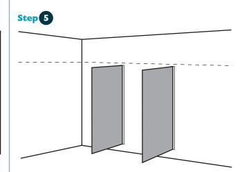
Place division panels into rear U-Channels with 4"x2" blocks underneath to make them level (wedges will be required).
