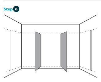
Fix side U-Channels (1795mm) flush with Datum and centred on marks. The U-Channels are predrilled. Ensure screws go into wall frame.
