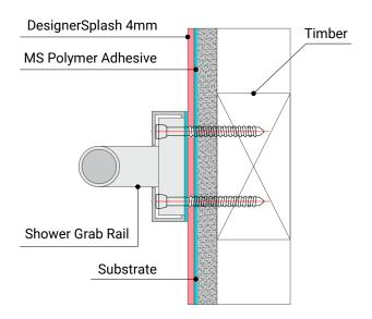
Where the panel is required to be waterproof, BRANZ recommends the following approach: Identify, mark, and predrill the fixing location. Before inserting the fixing, fill with sealant. Apply sealant to the back face of the plate or bracket before fixing through the DesignerSplash to the framing.
