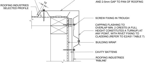
BARGE FLASHING DETAIL
