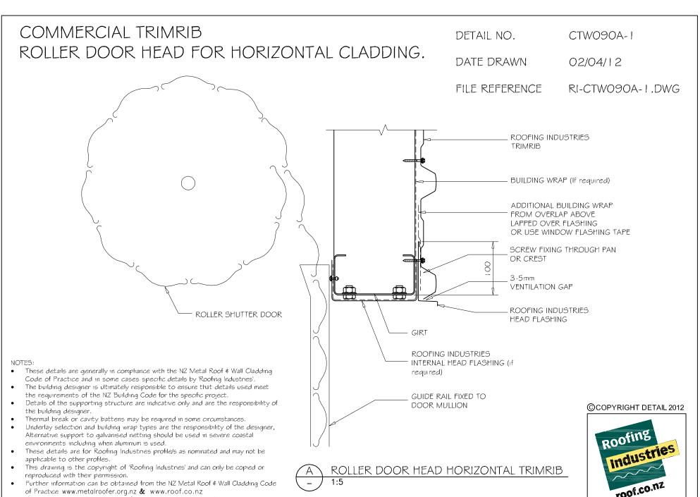
Where necessary adjust drawings for purlin battens or cavity battens.
