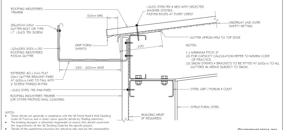
Alternative support to galvanised netting should be used in severe coastal
