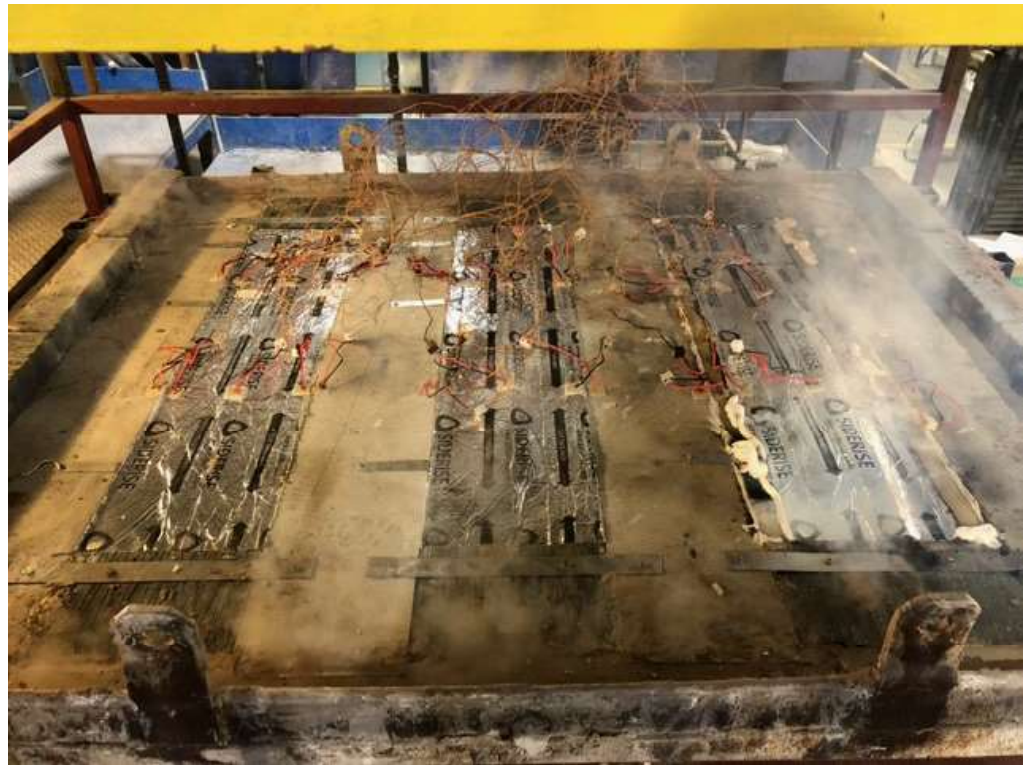
The unexposed face of the floor assembly after a test duration of 132 minutes
