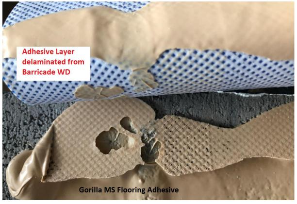
Masons Barricade WD Sealing Test
