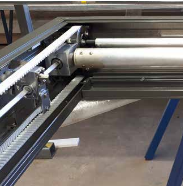
ROTATE MOTOR & RETRACT DRIVE SHAFT
