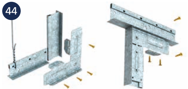
The XD10 securely joins two tier grid components at a 90° angle. Bend down tabs secure the Clip to the grid. Screws provide a structural connection.
