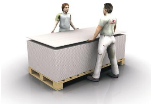
Figure 2 Whenever possible, lift the panel from the stack below rather than slide panel or drag off the stack. This will prevent damage by scratches to the lower panel.
